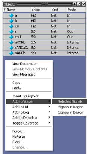
This should open up the **Wave** tab with all of the signals from the **fullAdder** module.
