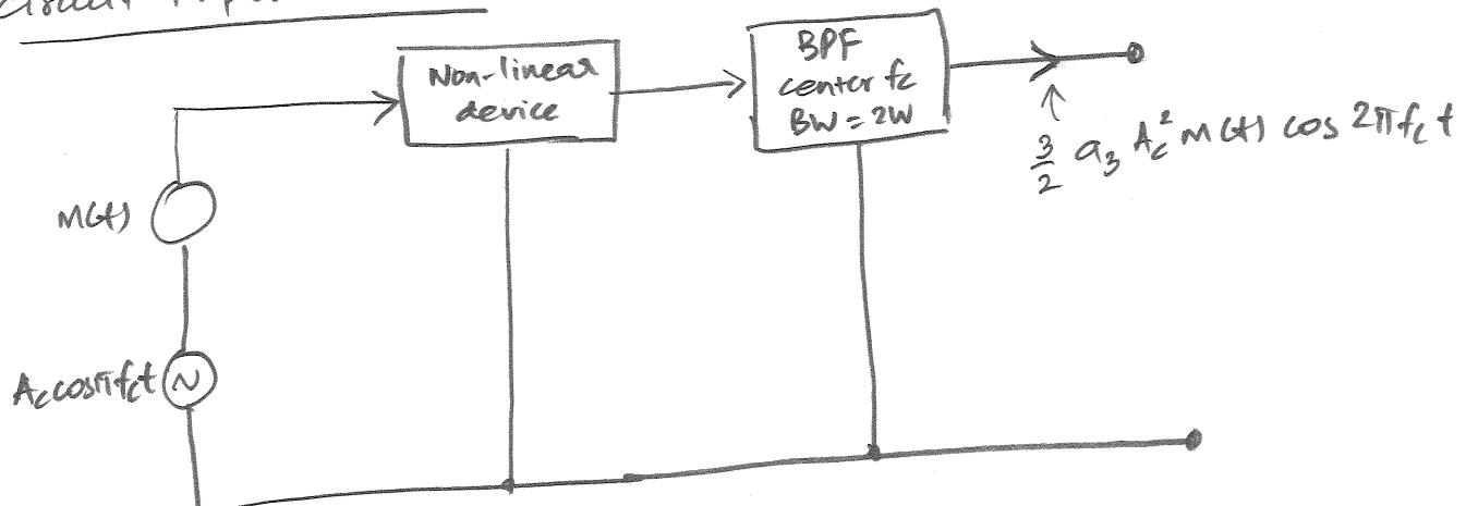
(b) To obtain an amplitude modulated signal, we need an additional sinusoidal signal added to the product modulated signal from part (a). This is achieved by using two branches as shown below. The first branch is same as the product modulator. The second branch has a constant input instead of a message signal.
