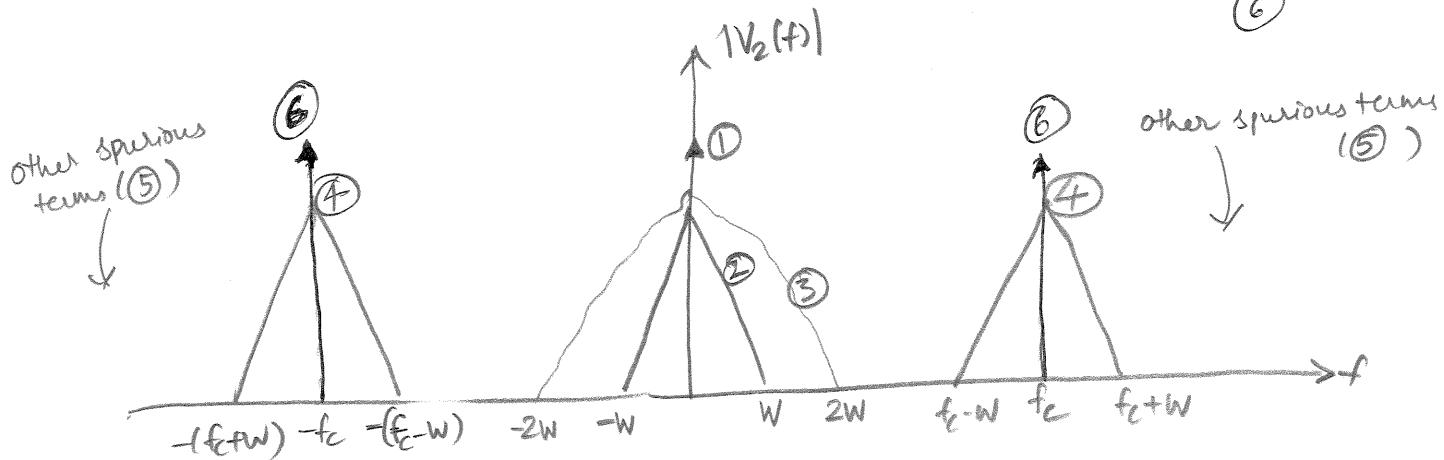
(b) Pass  $v_2(t)$  through a LPF of BW =  $W$  Hz
