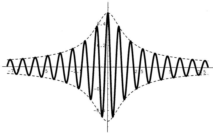
SSB (Lower Sideband) Signal =  $.5*(1/(1+t^2)*\cos[2*\pi*l*t]+t/(1+t^2)*\sin[2*\pi*l*t])$
