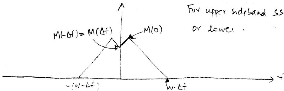
For upper sideband SSB with  $\Delta f \leq 0$  or lower ...  $\Delta f \geq 0$
