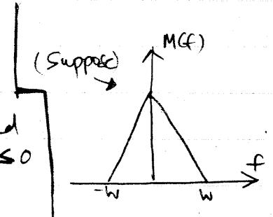
① For upper sideband SSB with  $\Delta f > 0$ , or lower sideband with  $\Delta f \leq 0$
