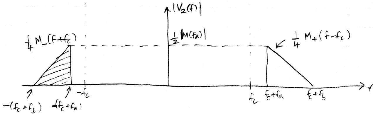
$$V_3(t) = V_2(t) \cos(2\pi(f_b + f_c)t)$$
