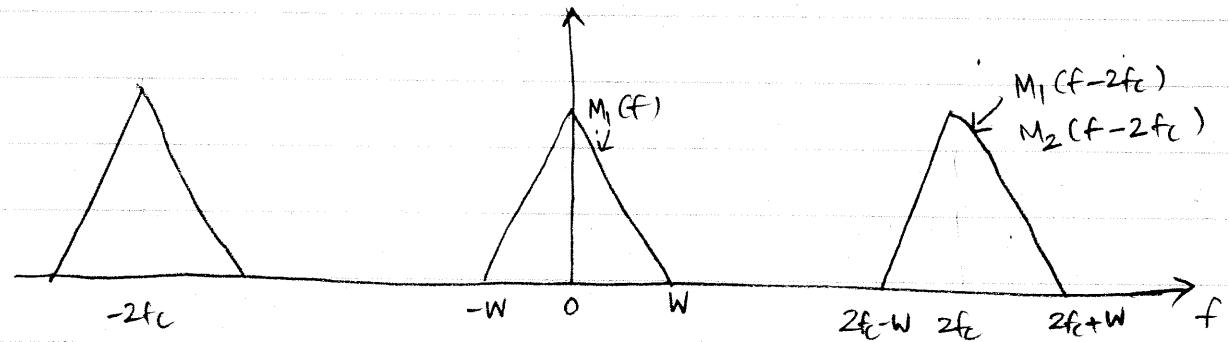
If  $m_1(t)$  and  $m_2(t)$  are band-limited to  $-W \leq f \leq W$  and  $2f_c - W \geq W$ , i.e.,  $f_c \geq W$ , then output of LPF is
