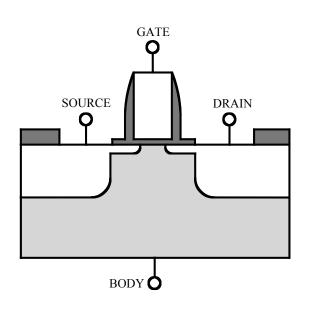
Tox scaling resulting in increased gate leakage caused by oxide tunneling
