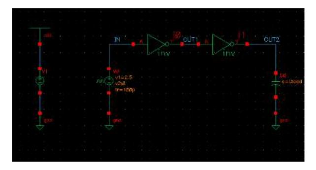
Figure 2: Final schematic of the testbench used to test our inverters.
