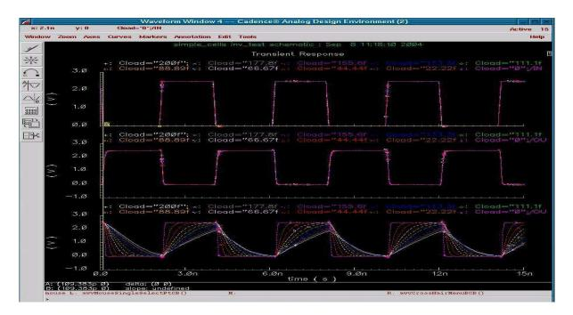
Figure 4: Parametric Analysis of the inverter testbench with output capacitance, Cload, varied from 0f to 200f.
