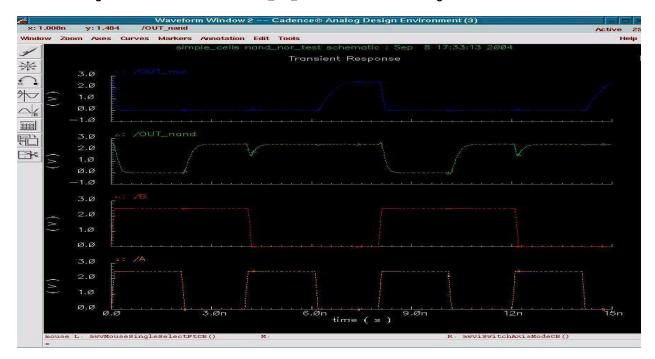
Figure 6: Output voltage waveforms for the nand\_nor\_test SPICE simulation.
