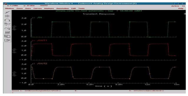
Figure 3: Voltage output waveforms from the inverter testbench.
