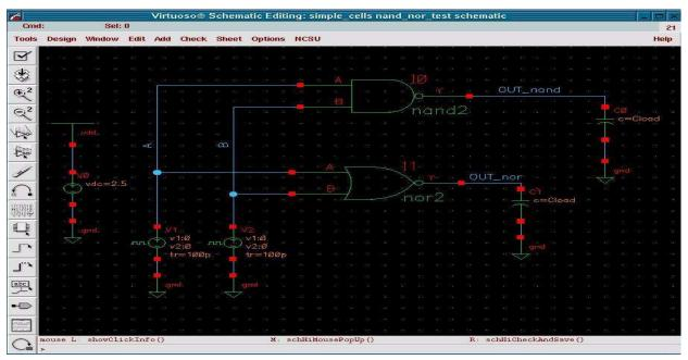
Figure 5: Schematic testbench 'nand\_nor\_test' to test NAND and NOR gates.
