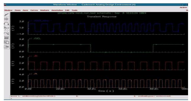
Figure 8: SPICE simulation results of mux\_nand\_nor\_test.
