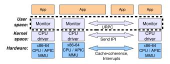
Figure 5: Barrelfish structure
