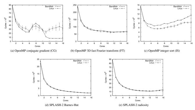
Figure 9: Compute-bound workloads on 4×4-core AMD (note different scales on y-axes)
