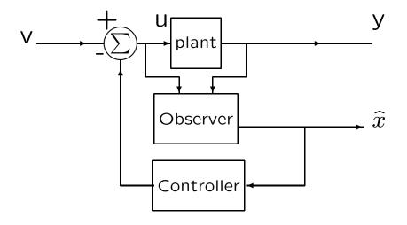
This is a powerful prototype for control system design in which the choices of controller and observer parameters can be made in a separated/independent manner.
