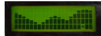
LCD Showing Openspace Distribution: Each column is an Openspace bin with height proportional to desirability of that direction
