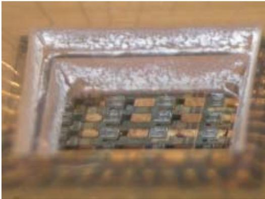
**Figure 7. Two-level Loctite™ encapsulation**
