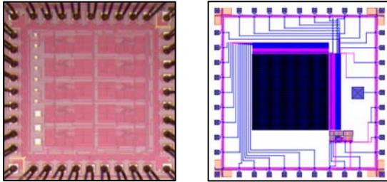
**Figure 2. Legacy amplifier design (left); new neurite outgrowth monitoring design (right)**
