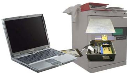
**Figure 5. Data acquisition system components and general setup**
