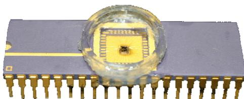
**Figure 6. Fully packaged and encapsulated chip**
