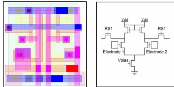
**Figure 3. Lay out of in-pixel NMOS-differential amplifier unit (left); schematic (right)**
