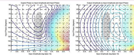
The contour plots of input and output phase and amplitude of MZI with SA are shown above. Best operation regions are indicated by the shaded areas where output is predominantly flat.
