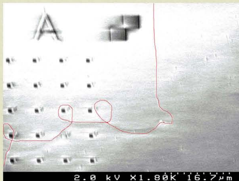
Figure 2: An SEM image of alignment markers on top of silicon. The path of the CNT is shown in red.
