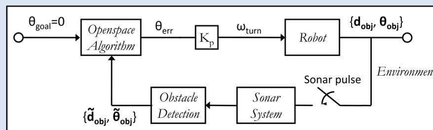
This figure details the flow of data in the real-time system. Once the *Openspace* evaluation function calculates the winner-take-all angle, a proportional controller adjusts the robot's movement accordingly. Then the sonar system and obstacle detection code re-evaluate the environment to provide feedback.
