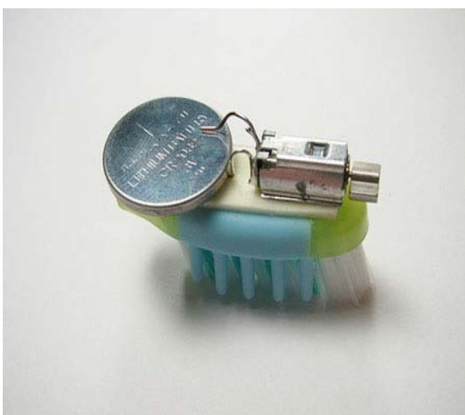
We used the model of a bristle bot to determine the movement of the "robots" in our simulations
