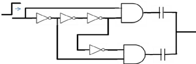
Fig. 3. Spike circuit: The circuit above will generate narrow spikes corresponding to each edge of the incoming signal.
