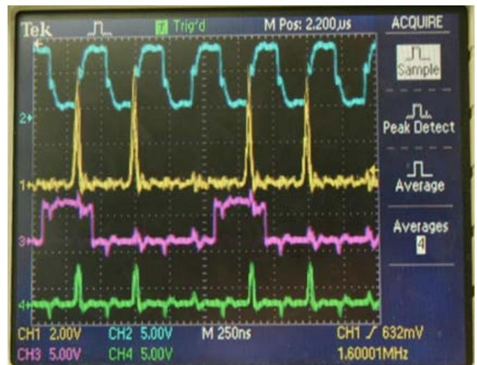
Fig. 7. A clean signal enters the receiver (110110). It is digitized and sent to the RAKE. A row of latches captures the data (not shown). The data is matched with the stored pattern and the RAKE outputs a
