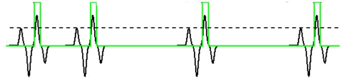
Fig. 4. A sequence of pulses and corresponding digitized output. In this example, the dashed line is the threshold level.
