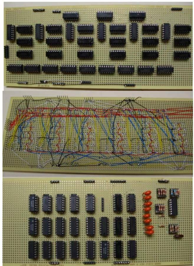
Fig. 9. The receiver and transmitter circuit board. Top, a portion of the RAKE receiver. Middle, the backside of the RAKE receiver. Bottom, the transmitter.
