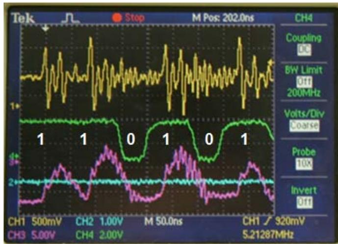
Fig. 8. The output of the transmitter is directly connected to the receiver. The RAKE is able to digitize the incoming signal to the correct pattern in spite of a high level of noise. Legend from top to bottom: incoming noisy signal, recovered digital pattern (output node of one latch), output of the comparator circuit, and the flat line is the threshold.
