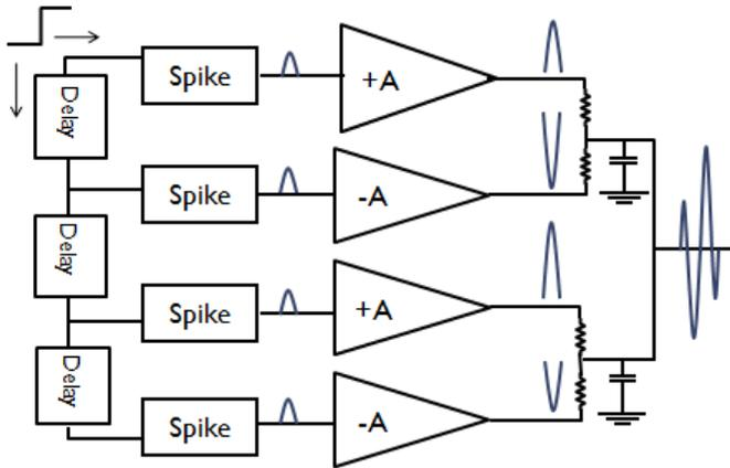
Fig. 2. Pulse Generator: The circuit above generates a sequence of pulses corresponding to each edge of the incoming signal. The Spike circuit is shown in Fig. 3. Each triangle represents an op-amp. Symbols +A and -A represent non-inverting and inverting configurations, respectively.
