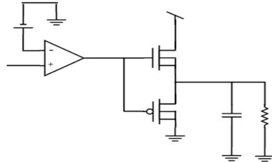
Fig. 6. Implementation of the comparator. The negative side of the Op-Amp is the threshold voltage which will be swept from 3 volts to 0.2 volts.
