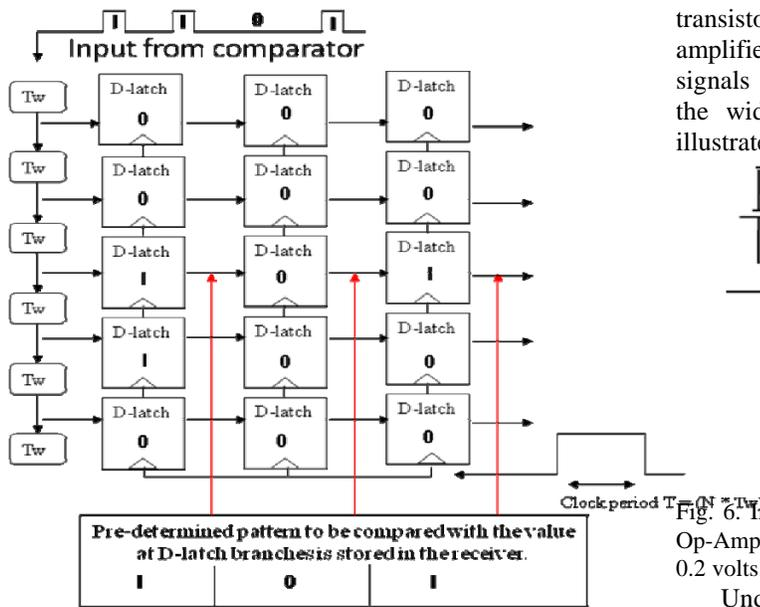
Fig. 5. RAKE receiver. The rake receives digital inputs from the comparator. These inputs move down the delay line on the left and are sampled by latches. The information moves right until it reaches the end and is discarded. There is an ongoing comparison to check if at any time data present in the latches matches the pattern. If so, the system will output logic value of ‘1’, if not logic value of ‘0’.
