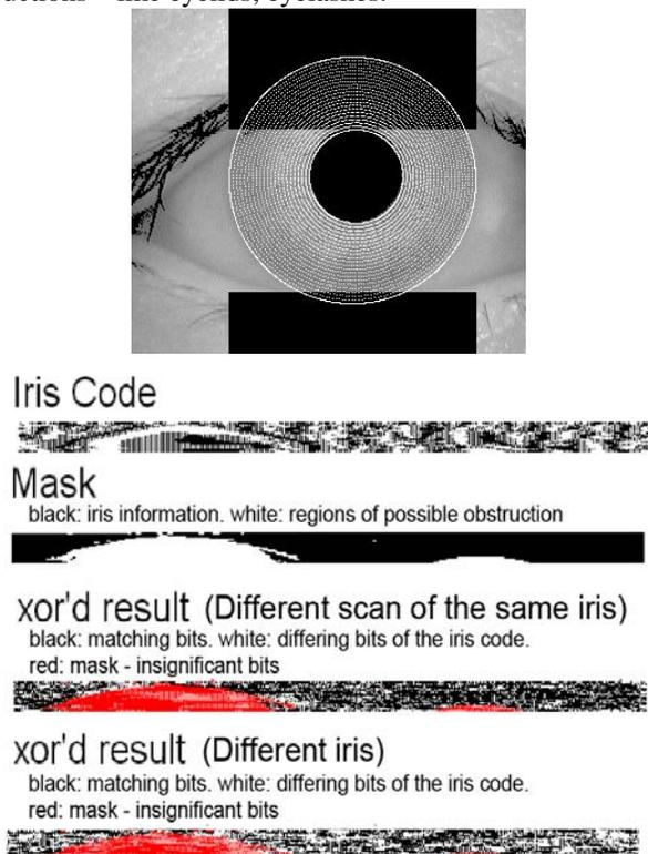
Fig. 2. Examples of a segmented iris and mask.
