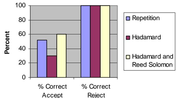
Fig. 3: Comparison of different error correction techniques used for XOR-ECC
