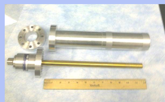
Figure 1. Coaxial cylindrical capacitor used to take measurements, unassembled.
