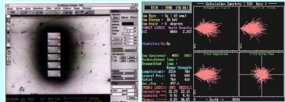
Gallium ions were incorporated into the SiC lattice using Focused Ion Beam (FIB) surface-modification.
