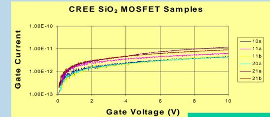
Current versus voltage measurements for several SiO<sub>2</sub> MOSFET gates on a SiC test chip from CREE industry. Collected using HP4145B and Interactive Characterization Software.
