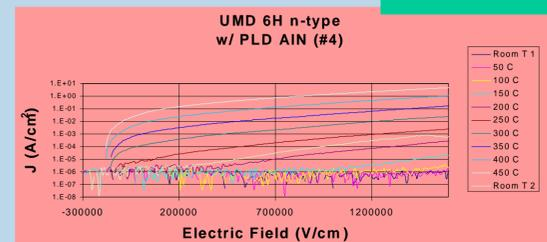
Current density versus electric field for TiN/AlN/SiC capacitor at varying temperatures. Collected using HP4145B and Interactive Characterization Software.
