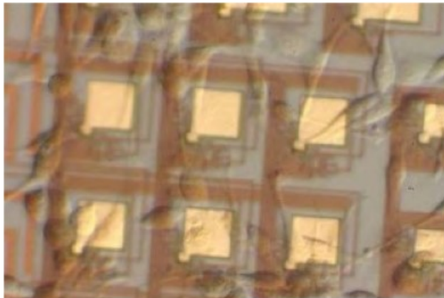
Heart cells on capacitance sensors
