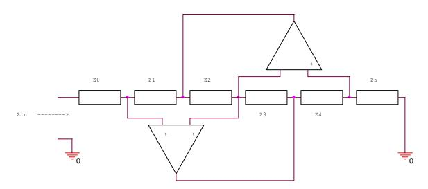
Choose Z2 and Z4 as equal capacitors of capacitance C and all other branches as resistors with equal resistance R.
