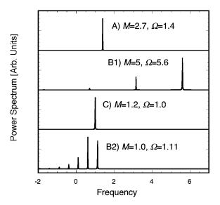
FIG. 6. Power spectra for r(t) for four representative points in the M vs  $\Omega$  plane for K=5. The four curves have been offset to separate them. The letter label of each curve indicates the corresponding region of Figs. 3 and 4. Curve B1 is close to the boundary of region A, and curve B2 is close to the boundary of region C.
