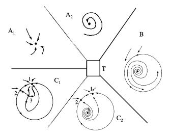
FIG. 4. Schematic phase portraits of the equilibria in various parts of parameter space surrounding the point T. The boxed region corresponds to the parallelogram of Fig. 3. For the phase portraits in this region the reader is referred to Ref. 15.
