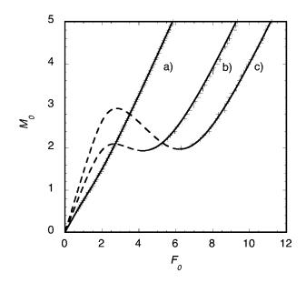
FIG. 2. Driving strength  $M_0$  vs force  $F_0$  for (a) K=1,  $\Omega=1$ , (b) K=5,  $\Omega=2$ , and (c) K=7,  $\Omega=2$ . The continuous curves are solutions of Eq. (6) with stable equilibria [according to Eq. (21)] shown as solid lines and unstable equilibria shown as dashed lines. The crosses are the results of simulations of Eq. (1) with 1000 oscillators for the cases in which the force approached a steady value.
