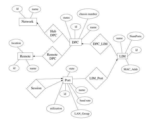
Figure 5.1: Entity-Relationship diagram for Configuration Management
