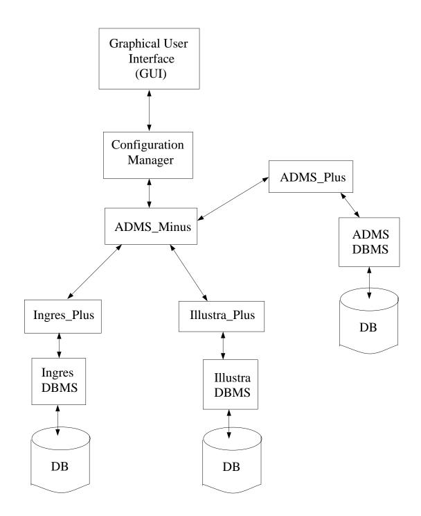
Figure 5.2: Configuration Management Architecture
