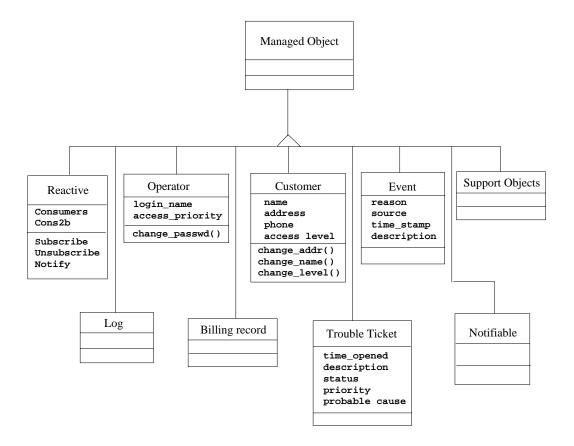
Figure 2.6: Managed Object Inheritance hierarchy
