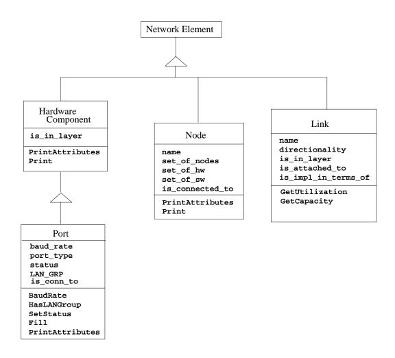
Figure 2.12: Specialization of the Network Element class
