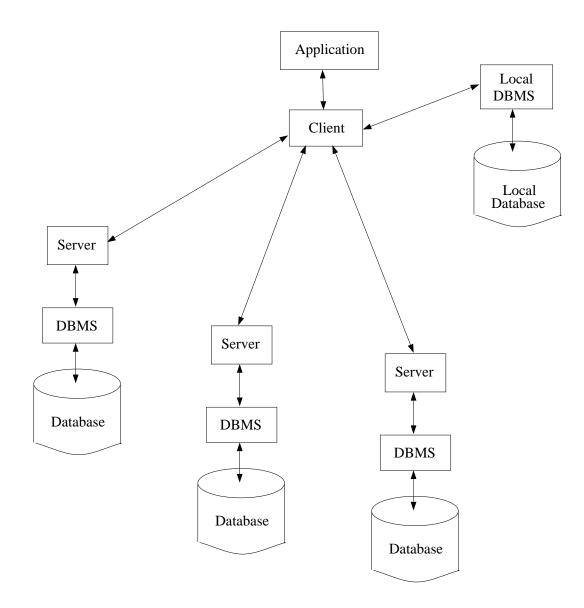
Figure 4.1: Database Integration Architecture
