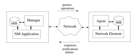
Figure 2.1: A typical Network Management System scenario
