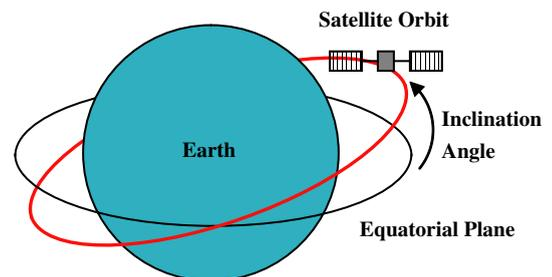
Fig. 4. Definition of a satellite's inclination.
