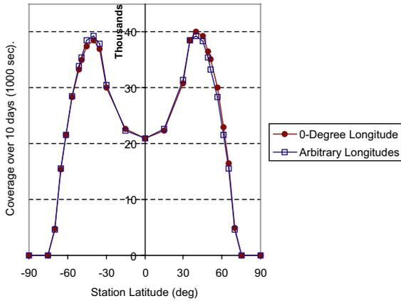
Fig. 5. Coverage for varying station [lat, long].
