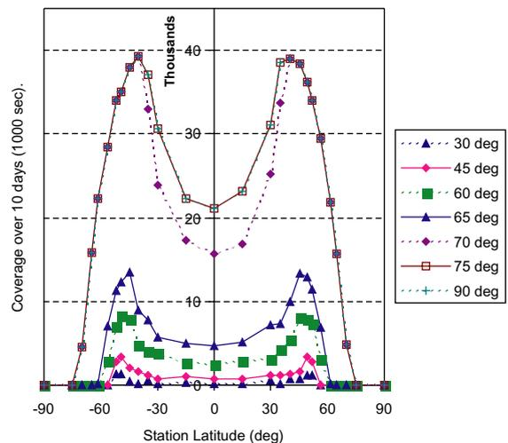
Fig. 7. Coverage for varying ISS antenna cone angles.
