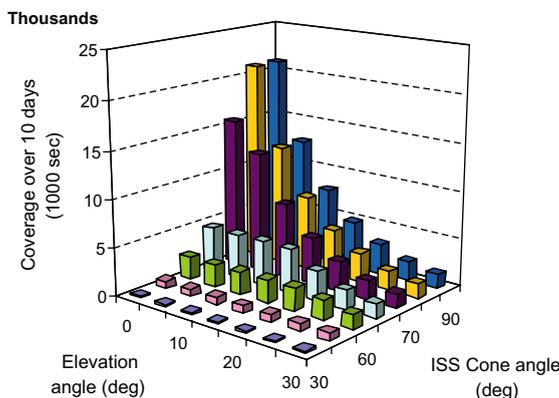
Fig. 8. Coverage for varying elevation angle and cone angle.
