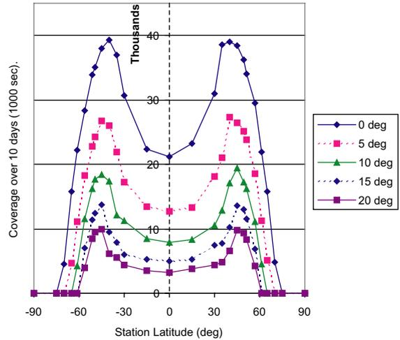
Fig. 6. Coverage for varying elevation angle.
