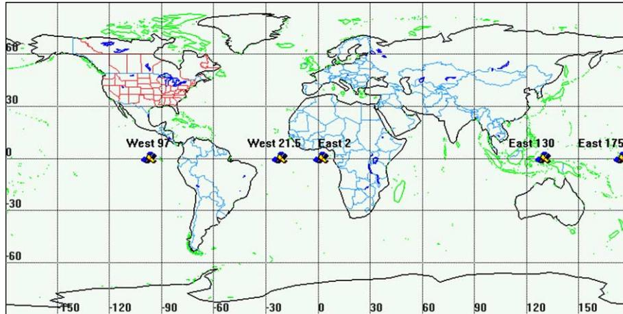
Fig. 10. Astrolink constellation at the five orbital positions.
