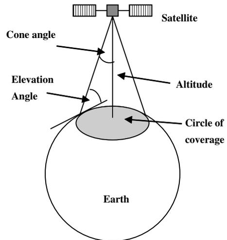
Fig. 3. Definition of cone angle and elevation angle.
