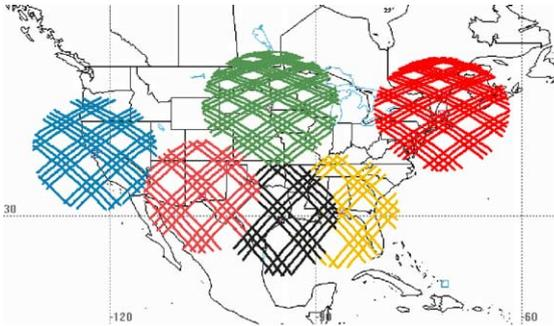
Fig. 9. Ground track of ISS with access to six US stations.
