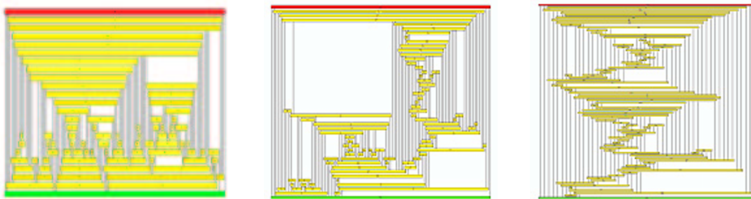
Figure 5.6: Visibility Representations of an 85-node triangulated planar graph for different st -orientations produced with PAR-STN( p ) ( p = 0, 0.5, 1 ).
