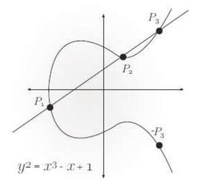
FIGURE 8.2: An elliptic curve over the reals.
