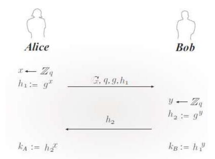
FIGURE 10.2: The Diffie-Hellman key-exchange protocol.
